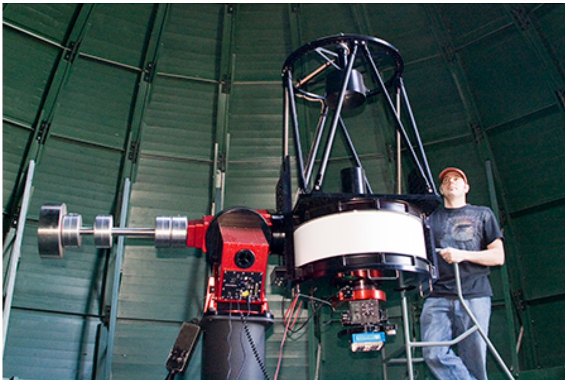
Arron Shiffer (BS Physics & Astronomy, 2009) prepares for a night of observing with the Lutz telescope and the Apogee Instruments 1k x 1k CCD science camera (blue box in the photo).
